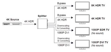
**Note**: If the source resolution is downscaled and converted to **1080P DVI** according to the EDID of display devices, it will be output without sound on TV.
