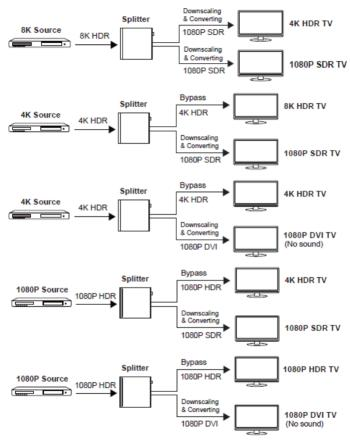
Note: If the source resolution is downscaled and converted to 1080P DVI according to the EDID of display devices, it will be output without sound on TV.
