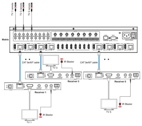
Figure 1: IR connection diagram (Matrix end)
