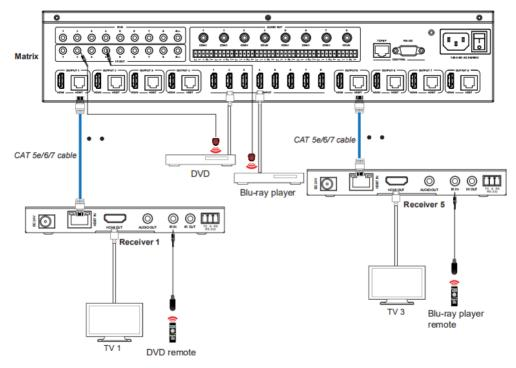
Figure 2: IR connection diagram (HDBaseT Receiver end)
