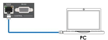
Step 3: Input the current IP address of Matrix into your browser on the PC to enter the Web GUI page.
