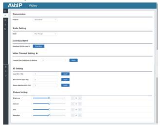
**Transmission Protocol:** You can select "UDP unicast" or "UDP multicast" (UDP multicast by default).
