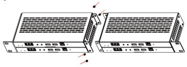
**Step 3:** Fasten screws between two 1U rack panels, so that four products are mounted in a 1U rack, as shown in the figure below:
