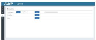
Click "Browse..." to import the upgrade file and click "Update" to start the upgrade. There will be a progress bar prompt during the upgrade process. When the progress bar reaches 100%, it indicates the upgrade is successful, and the device will be restarted automatically.
