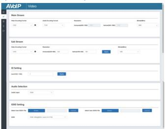
**Mainstream:** You can configure Video Encoding Format, Audio Encoding Format, and Bitrate. Video Encoding Format supports H.264 and H.265 (H.265 by default). Audio Encoding Format supports PCM and AAC (PCM by default). Encoding Resolution cannot be set, it follows the input resolution. The default Bitrate is 8Mb/s.
