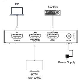
**Note:** When eARC function is turned on, the audio signal of Amplifier is the audio returned from 8K TV. When eARC function is turned off, the audio signal of Amplifier is from the HDMI input source.
