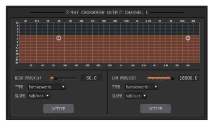
ACTIVE: When pressed, you will activate/inactivate the frequency filter (High Pass or Low Pass). The activation can be realized by clicking the green letter A at the 2-WAY module on the HOME page. The difference is that clicking the letter A will activate/inactivate the High Pass Filter and the Low Pass Filter simultaneously while clicking an ACTIVE button on the setting page will only activate/inactivate the corresponding frequency filter.
