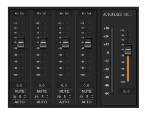
**FADER:** Each MIC input channel has a fader to adjust its signal level. It controls the mixed volume on the input channel.
