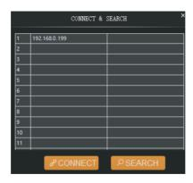
**Step 5**: Choose the audio processor's IP address and click CONNECT. Then the processor will relate to the host computer. After connection, the CONNECT & SETUP box (see the figure below) will pop out. You may close it directly if no such operation is needed.
