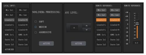
**LOCAL INPUT:** This shows source signals available to access the AEC process.AUTOMIXER refers to mixed signals after the AUTOMIXER process.
