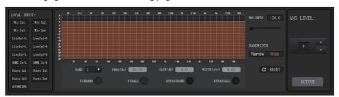
**MAX DEPTH:** The maximum amount of gain the module allows to reduce, with a scaleof [-20.0, 0.0] dB.
