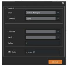
All RS-232 control commands, such as Scene Management, I/O Control, Modules' Configuration, and Device Information, can be found on the page. The command code will be listed at the bottom of this page once you have selected the Type, Command, Channel, and from the drop-down box and entered its value.
