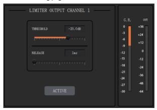
**THRESHOLD:** This shows that level signals above the threshold will be attenuated, with a scale of[-60.0, 0.0] dB.
