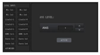
**LOCAL INPUT:** This shows source signals that are available to access the ANS process. AUTOMIXER refers to mixed signals after the AUTOMIXER process.
