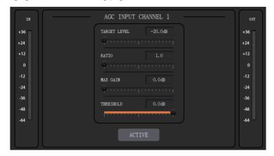
**TARGET LEVEL:** The desired output signal level, with a scale of [-20.0, 0.0] dB. **RATIO:** The compression ratio for signals above the target level, with a scale of [1.0, 20.0]. Suppose the value sets to 2.0, signs above the target level will be reduced to  $\frac{1}{2}$  of the original.
