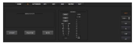
**SENSITIVITY:** Indicates the sensitivity level of the input signal, which could be adjusted to ensure the sensitivity on the input channel is adaptable to the MIC or linear input (function reserved).
