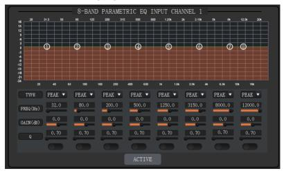
**TYPE:** Provides 3 types of band/filters, with High Pass, Low Pass, and Peak optional. **FREQUENCY:** In High/Low Pass Filter, it means the cut-off frequency of the EQ band; In Peak Filter, it means the center frequency point of the EQ band, with a scale of [20, 20000] Hz.
