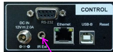
Audio connector for IR extender
